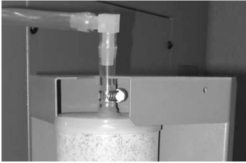
Use clamp on each end of filter to prevent leaking. Do not overtighten.
