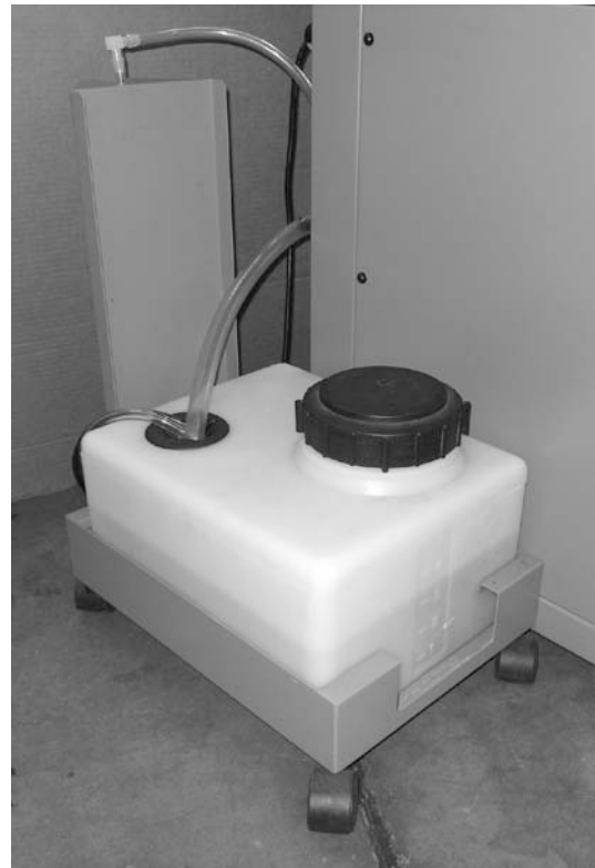
Finger-tighten the Water Supply and Drain connections to chamber. Plug pump wire into receptacle, turn clockwise to lock. Drain tube must not be submerged in the water. Installation behind chamber is not recommended because it may block the air vents.
