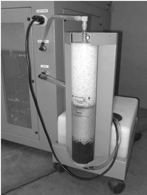
Finger-tighten the Water Supply and Drain connections to chamber. Plug pump wire into receptacle, turn clockwise to lock. Drain tube must not be submerged in the water. Installation behind chamber is not recommended because it may block the air vents.
