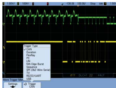
Capture long streams of serial data and gain fast insight into the problem with real-time hardware-based serial decode for I 2 C, SPI, CAN, LIN, FlexRay, RS232/UART and USB.
