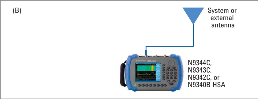
Figure 1. Spectrum analyzer configurations for measuring wireless interference (a) using a directional coupler and (b) using direct connection to the antenna
