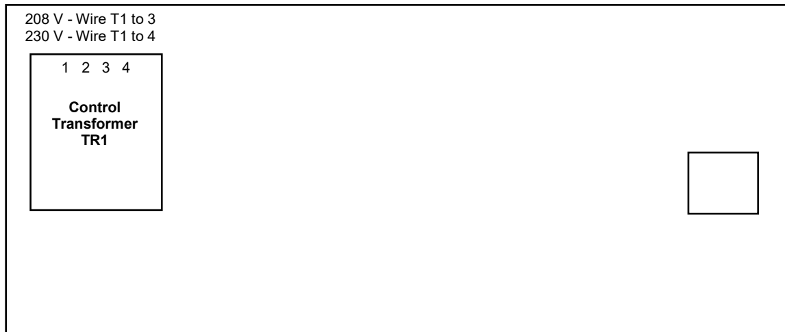
Figure 2-1 – Location of Input Configuration Terminals on the Electrical Sub Panel
