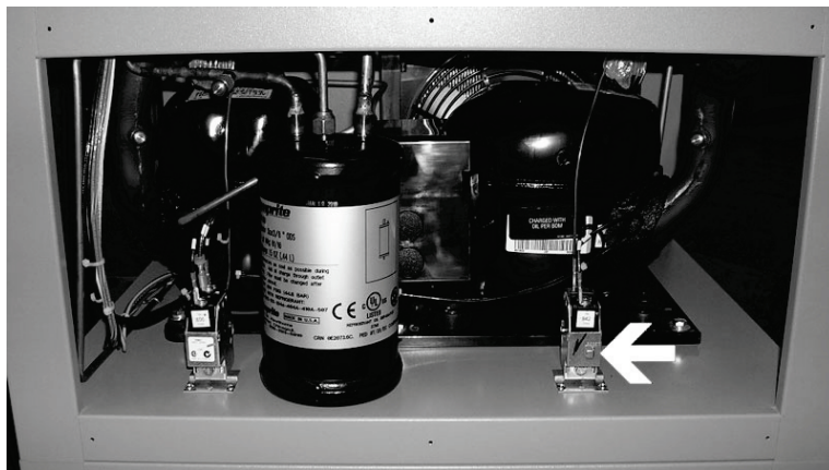
Figure 9.1 – PS2 Pressure Switch Reset Button (lower rear panel removed)
