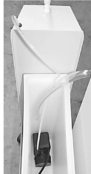
Pump placement in water tank.
