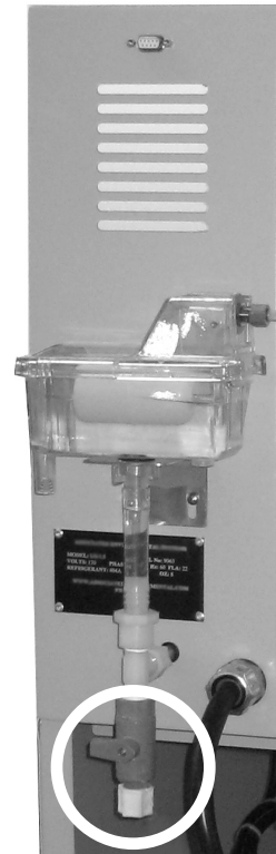
Figure 8-1 – Humidity Drain Valve (shown in the closed, or normal operating position)
