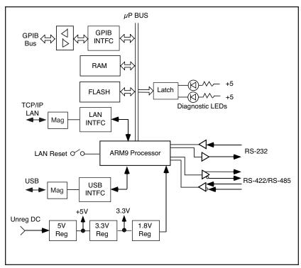
Figure 4-3 9009 Block Diagram
