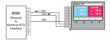
Figure 2-7 RS-232 Connections to a Watlow F4T
