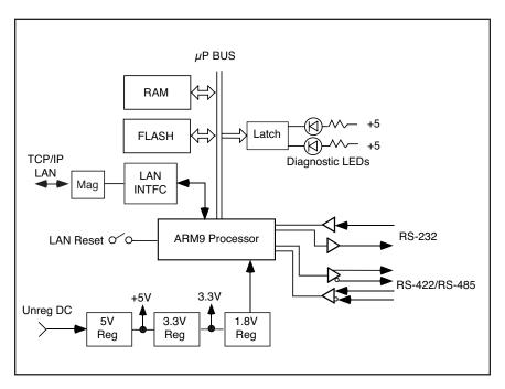
Figure 4-2 9099 Block Diagram
