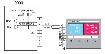
Figure 2-10 9099 RS-485 Connection to an F4T Controller
