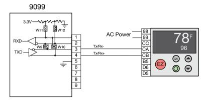
Figure 2-9 9099 RS-485 Connection to an EZ-Zone Controller
