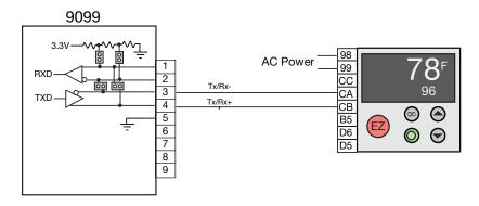
Figure 2-8 9099 RS-485 Connections to an F4 Controller
