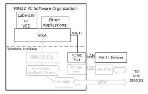
Figure 3-2 VISA to VXI-11 Communication Path
