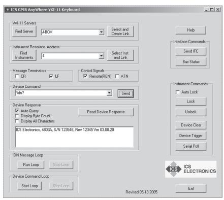
Figure 3-3 VXI-11 Keyboard Program Panel
