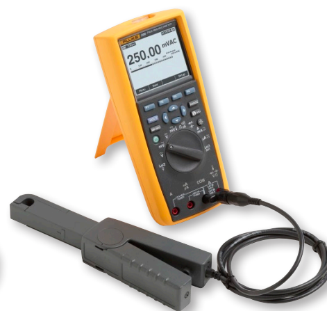
Figure 5: At 10 mV/A, a reading of 25 amps displays 250 millivolts.
