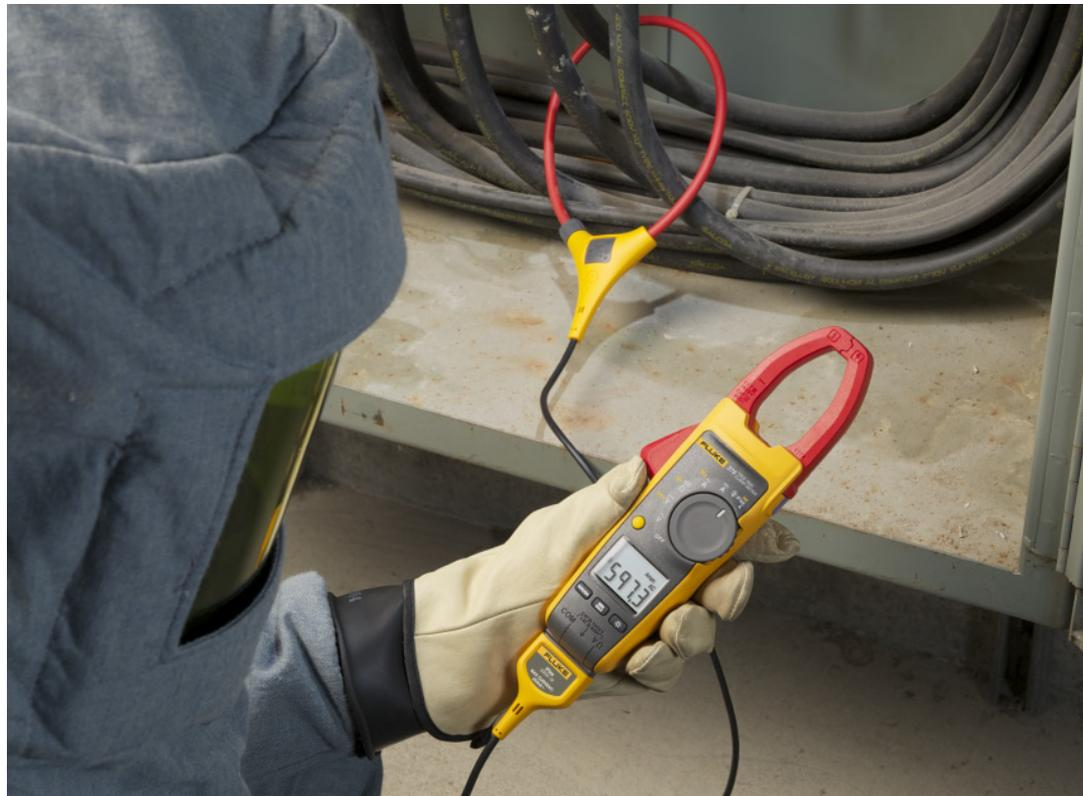
Choose a clamp meter rated to meet the electrical environment you'll be working in, as well as the resolution and accuracy of measurement you'll need for your testing.
