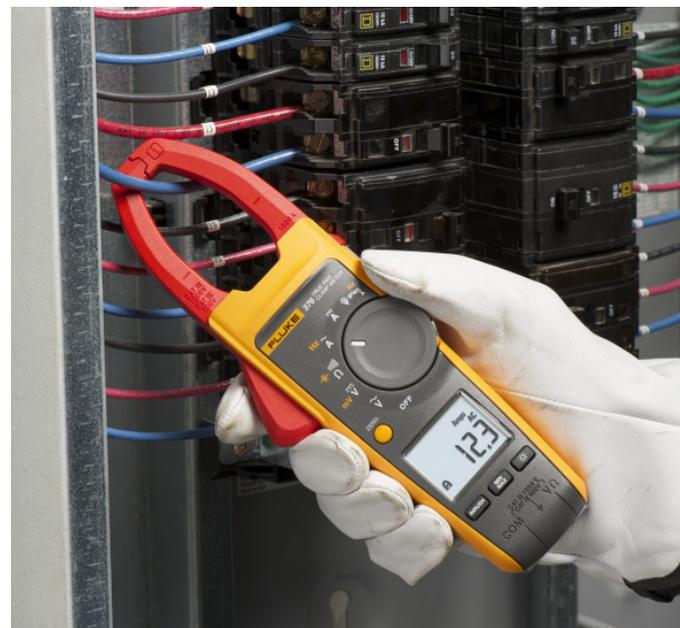
Measuring current with a clamp meter.
