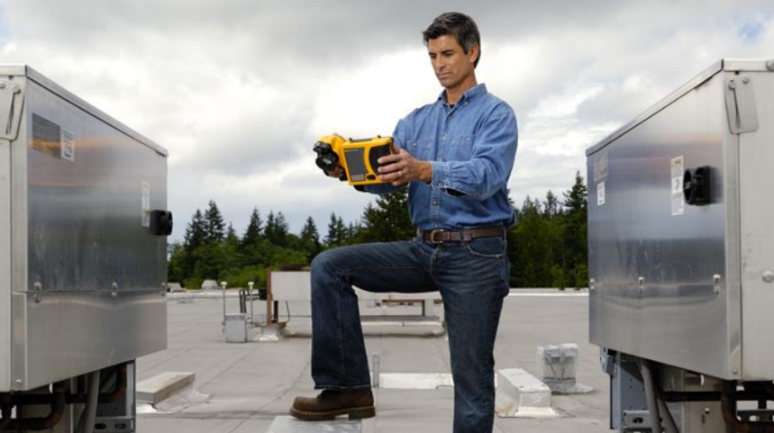
Figure 3. Figure 3: Qualitative measurements are fast for ducting, but accurate, quantitative measurements require compensating for reflectivity.
