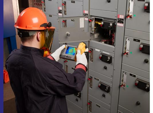
For troubleshooting, taking a thermal image of a malfunctioning unit can often identify the source of the problem electrical hotspots can tell you which phase or connectors to check, motor hotspots can narrow it down to bearings, and so forth. Then, after repairs, follow up with another thermal image and verify that the component is no longer overheating—or that something else isn't now overheating, instead.
