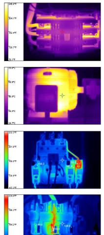
you can also change the emissivity or temperature range, to better analyze the results. That means you don't have to get the perfect image on-site, which is a big time-saver.
