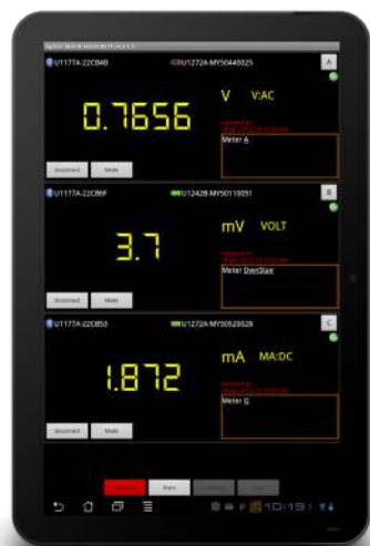
Figure 5. Up to three multimeters measurements with the Keysight Mobile Meter
