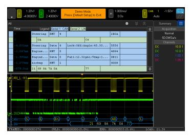
Figure 1: Capturing and decoding a CAN and LIN serial bus simultaneously on a Keysight InfiniiVision X-Series oscilloscope.
