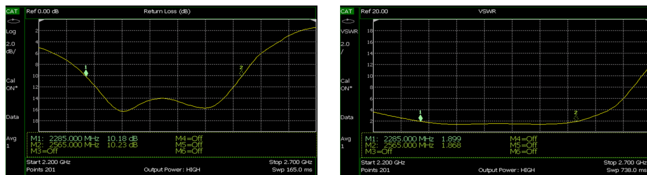
Figure 5a and 5b. Frequency response measurement of a panel antenna showing (a) return loss (dB) and (b) VSWR
