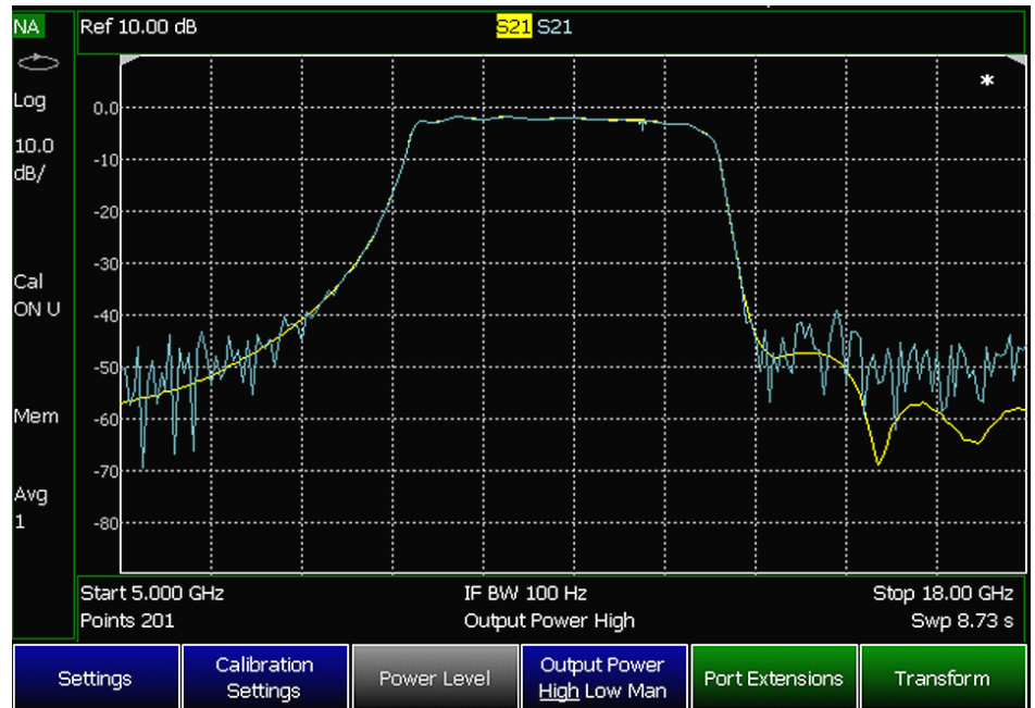
Figure 6. Measurement comparison of a 13-GHz band pass filter response using the High Output Power setting (yellow) and the Low Output Power setting (blue) on FieldFox
