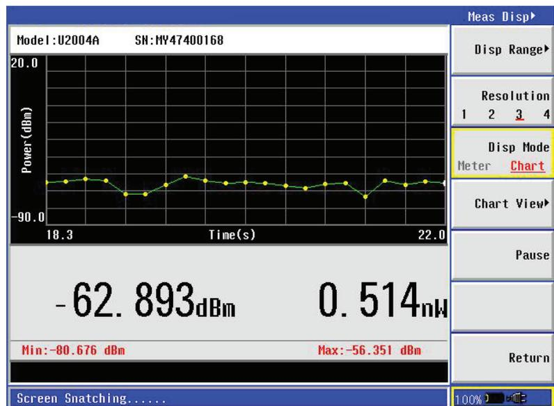
Figure 17. Measurement display in chart format
