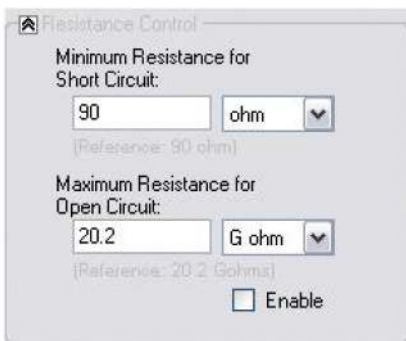
Perform short- and open-circuit testing through the resistance control capability.
