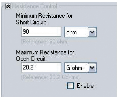
Perform short- and open-circuit testing through the resistance control capability.
