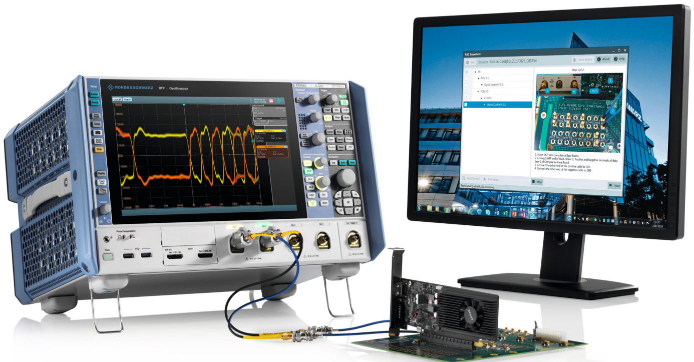
Automated PCI Express compliance test
