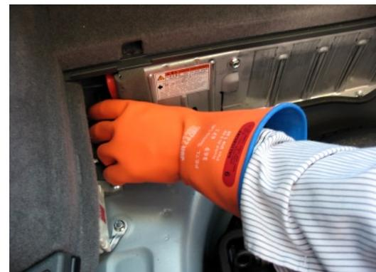
After putting on insulating gloves, the technician disconnects and removes the battery service plug. 2007 Toyota Prius hybrid shown.
