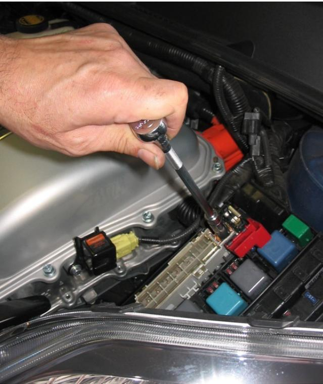
After turning the vehicle off, the technician disconnects the vehicle's auxiliary 12 V battery to ensure that the HV battery pack is mechanically isolated. The battery of this Toyota Prius can be disconnected from inside the main fuse/relay box.
