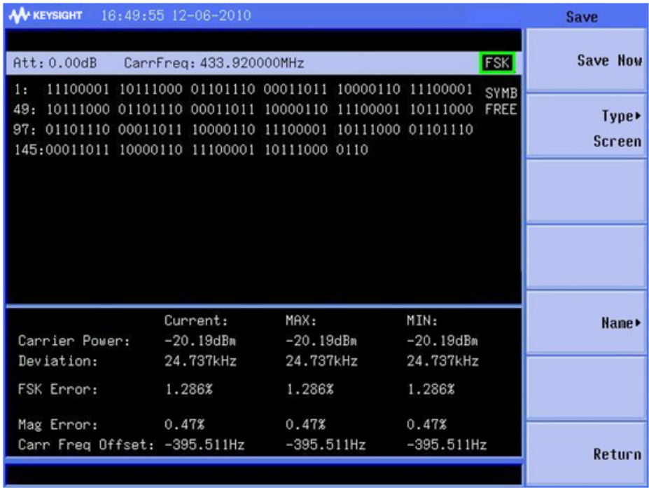
Figure 12. FSK demodulation – symbol view
