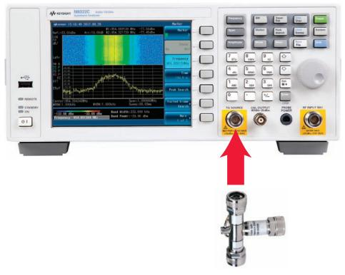
Connect the OPEN and TG SOURCE as shown. Once connected, press [ENTER] to continue, or [ESC] to abort.
