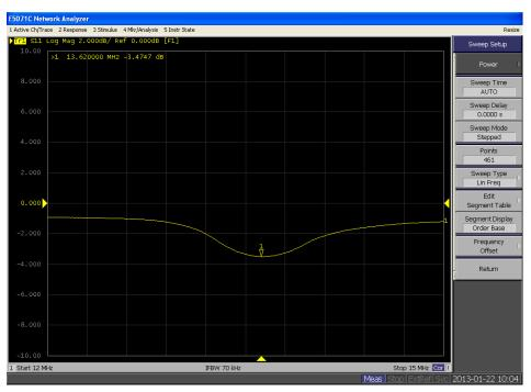
Figure 6. Return loss result measured with E5071C ENA
