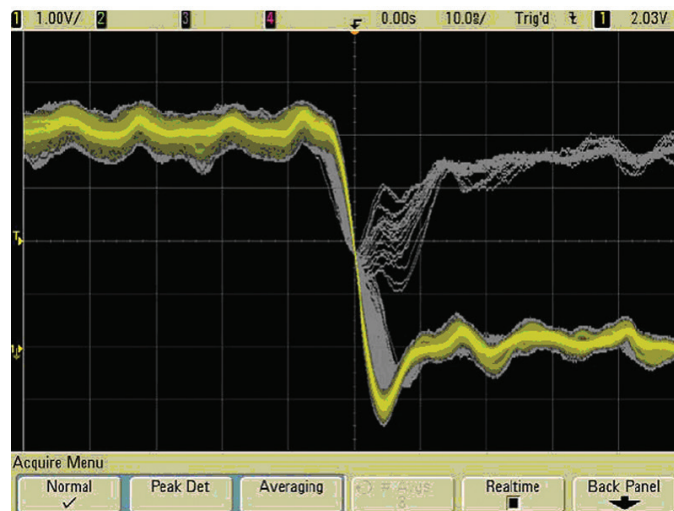
Figure 19. An infrequent glitch caught on a Keysight InfiniVision 6000 Series oscilloscope
