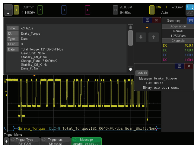
Figure 3: CAN-dbc symbolic decode and trigger.
