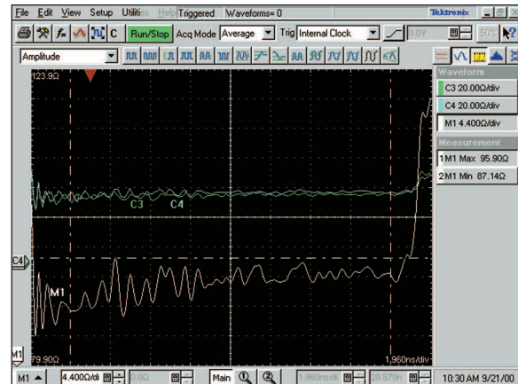
Figure 17: USB 2.0 impedance measurement, within specifications
