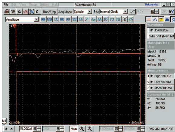
Figure 18. USB 2.0 impedance measurement, outside specifications (mask displayed)
