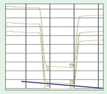
Poor low frequency S-parameter data from VNA using only couplers leads to DC-extrapolation errors and a slope in results for 25 ohm section. Noise impact on DC extrapolation causes wide variation in impedance results.
