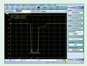
High quality low frequency S-parameter data from VNA with bridge/coupler hybrid architecture minimizes DC-extrapolation errors and gives accurate flat results with no observable variation due to noise effects.
