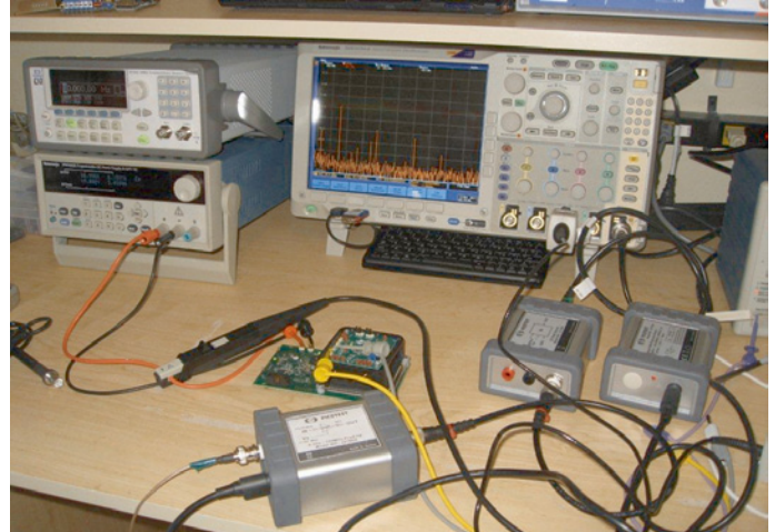
Figure 3. Test setup for measuring the charger including a Mixed Domain Oscilloscope, voltage and current probes, laboratory-grade power supply, and signal injectors.
