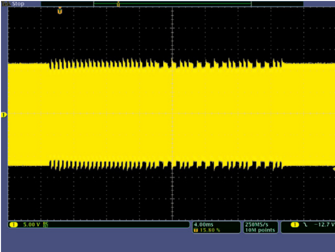
Figure 10. Primary coil voltage measured with the TDP0500 Differential probe.
