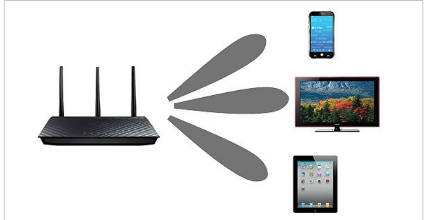
Figure 5. Simplified, beamforming focuses resources towards particular devices
