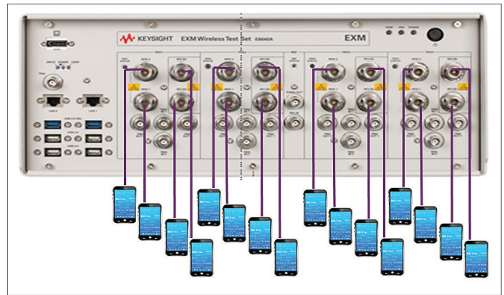
Figure 3. As shown here, the EXM permits the connection of up to 16 single-antenna DUTs
