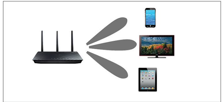
Figure 9. In simplistic terms, beamforming is a technique used to aim a signal directly at a target rather than broadcasting it to a wide area
