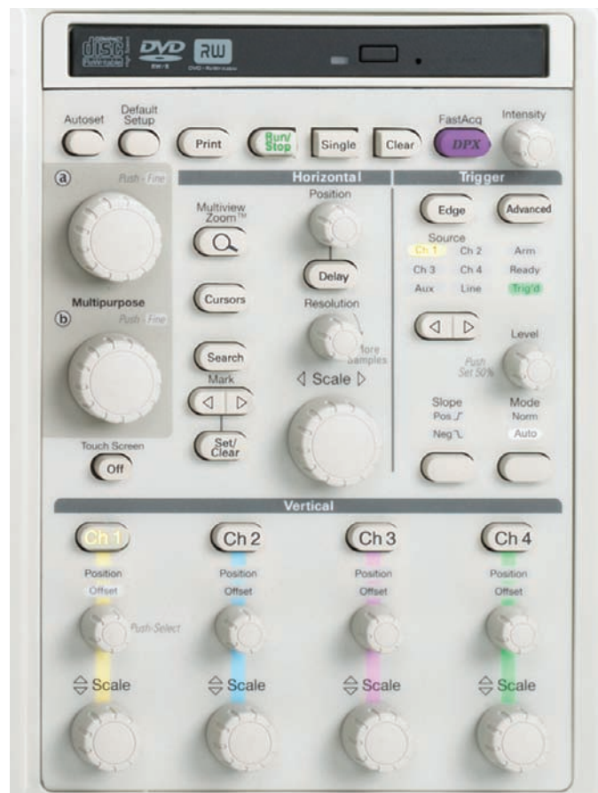
Figure 20. Front-panel control section of an oscilloscope.
