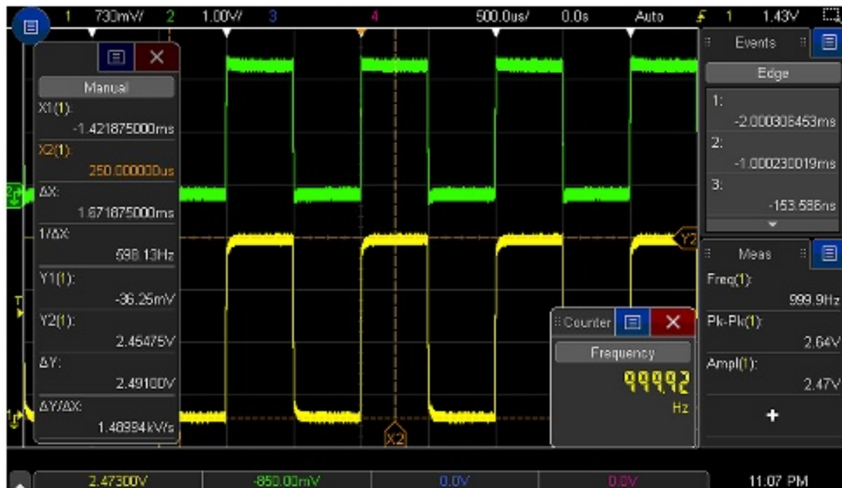
Figure 3. Side bar with movable docks allows information to be placed on the screen precisely where you want it for documentation.
