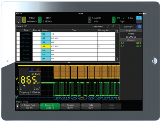
Figure 38. Tablet virtual front panel control.
