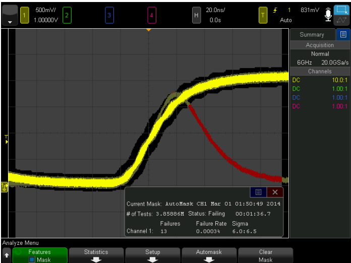
Figure 40. Limit testing of infrequent glitch.
