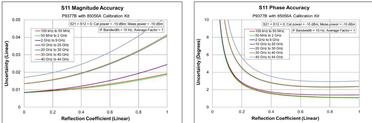
**Table 5. P9377B with N4693D electronic calibration (ECal) module with Option 0DC**
