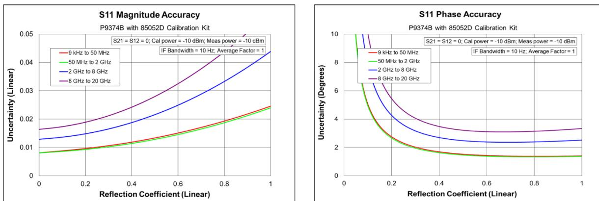
**Table 3. P9370B to P9374B, P9382B, P9384B with N4691D electronic calibration (ECal) module with Option 0DC**
