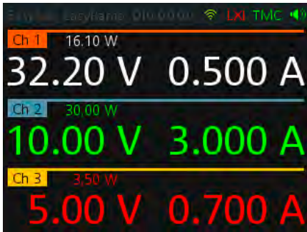
The different operating conditions are indicated by colors (example: R&S®NGE103B).
