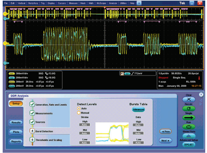
Figure 57. Advanced DDR analysis tools automate complex memory tasks like separating read/write bursts and performing JEDEC measurements.
