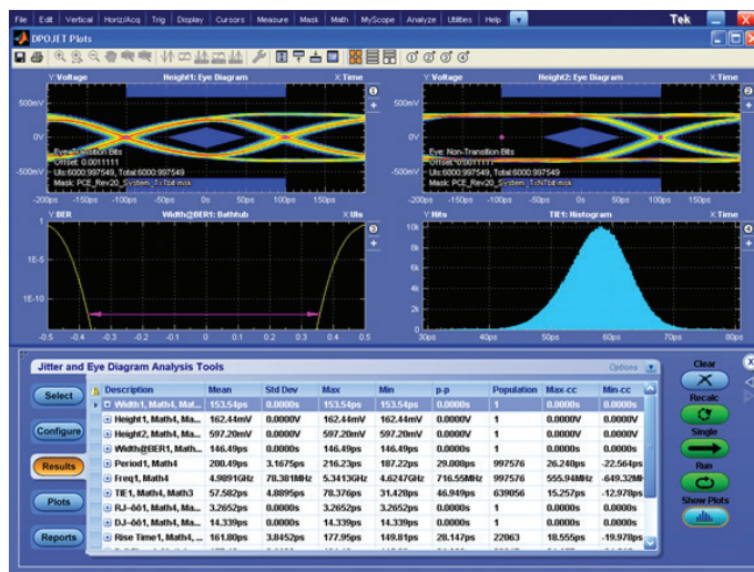
Figure 54. Analysis software packages are specifically designed to meet jitter and eye measurement needs of today's high-speed digital designers.
