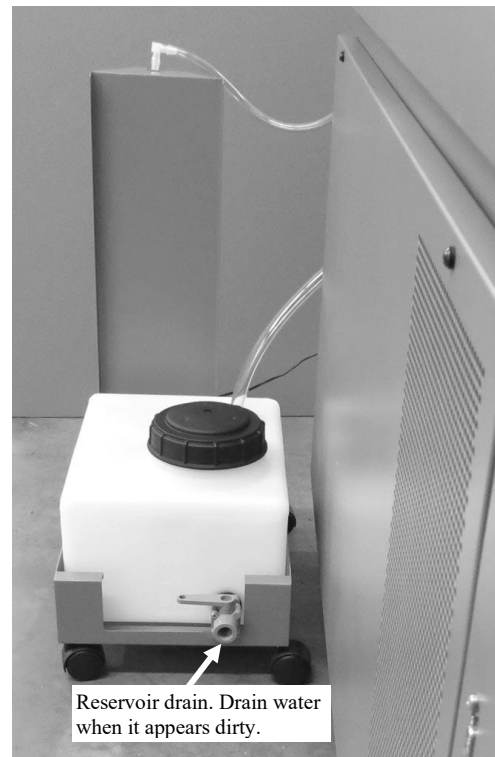
Figure 7-1 – Reservoir Drain Valve
